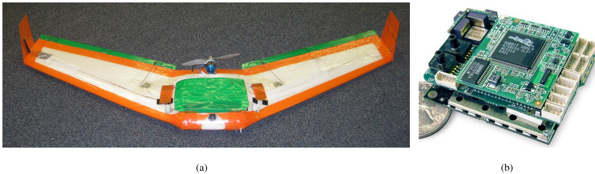
Fig. 10. (a) Small UAV used for testing. (b) Autopilot used for control.
