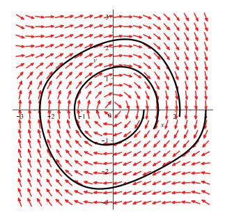
A compact region R is form by these orbit segments and the pieces of the x-axis between each of their first and second intersections with the x-axis.
